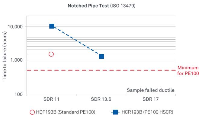
**Figure 2:** Notched Pipe Test ISO according to ISO13479 with varying wall thickness. Test covered 110 mm pipes of varying wall thickness with constant notch depth of 2.1 mm tested in hydrostatic pressure test at 920 kPa/80°C.
